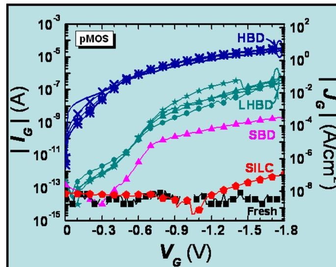
**Finding:** Degradation mechanisms induced by either EM-like pulse voltage stressing or DC stress the same.
