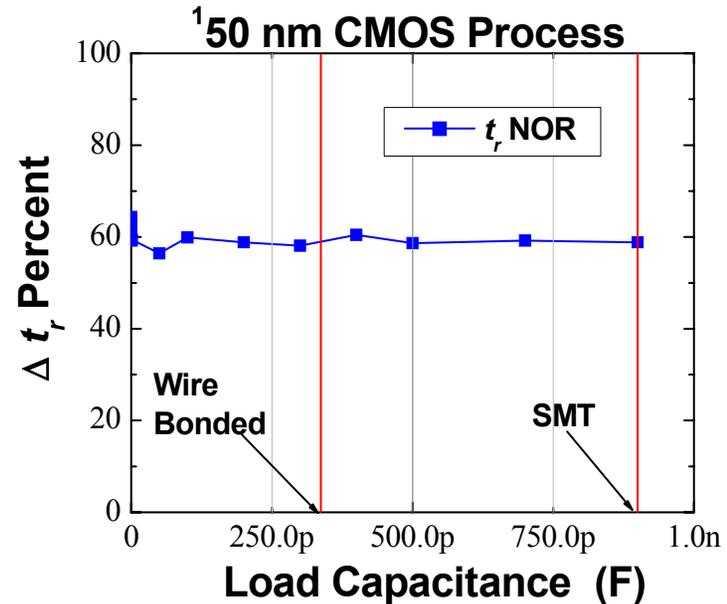
$\Delta t_r$  is within standard deviation when comparing wire bonded NAND circuit and SMT NAND circuit.
