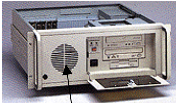
Shielding wall with opening for audio speaker
