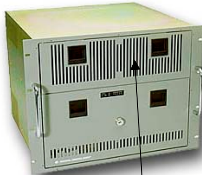
Opening for air ventilation
