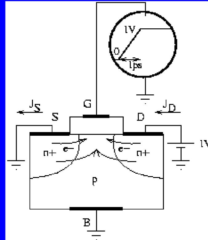
Results give I-V and Potential, Charge Concentrations, Current Densities inside device.
