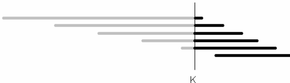
Fig. 5. This figure shows a beam which is in the process of formation but which has an initial contraction ( $\left[\frac{dz}{ds}\right]_0 < 0$ ) due to a velocity tilt imposed at the cathode.
