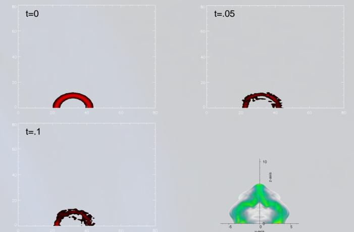
Example of current loop disintegration in a 64 x 64 x 16 grid-point simulation domain. At the lower right is the desired ideal MHD evolution from Ref. [2].
