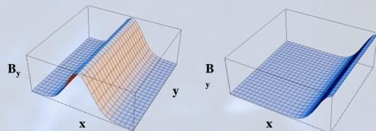
A test for conducting boundary conditions: Send a single Alfvén wave packet toward conducting wall and observe reflection
