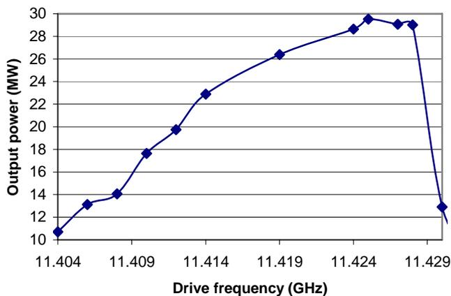
Fig. 5. Bandwidth curve for the 1-1-2-2 design (alpha=1.2)
