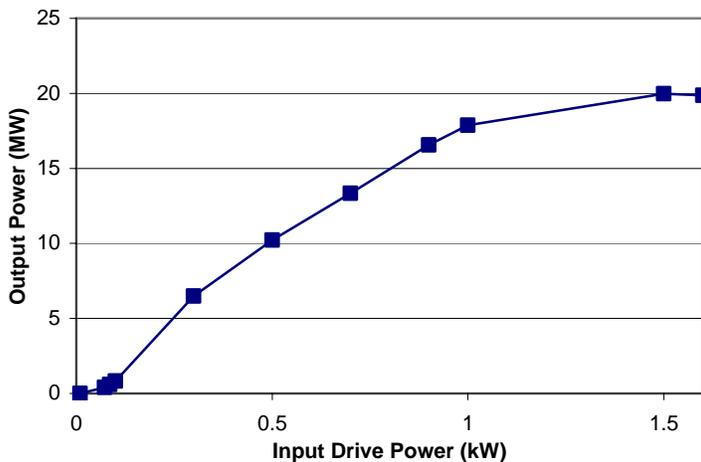
Fig. 8. Output power vs. the input drive power ( $\alpha=1.0$ )
