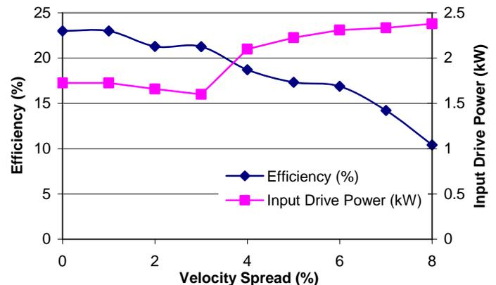
Fig. 6. Dependence of efficiency on axial velocity spread for  $\alpha=1.0$
