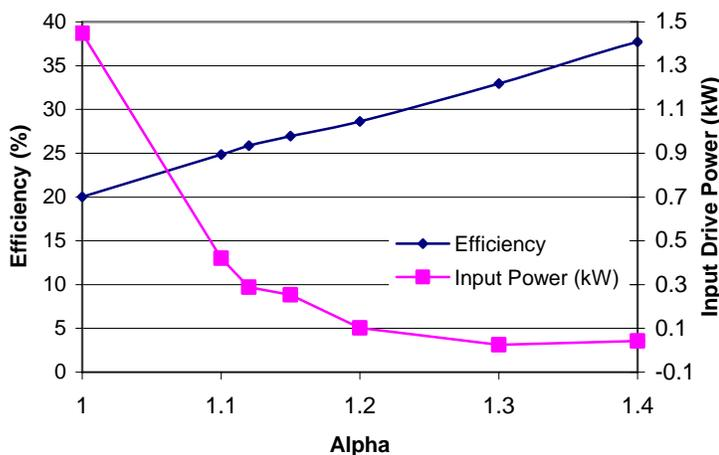
Fig. 4. Dependence of efficiency on velocity ratio
