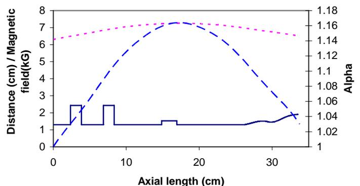
Fig. 2. Layout of a four-cavity frequency-doubling gyrokylystron circuit. Dotted lines represent the optimal magnetic field profile and the dashed lines represent the evolution of the average velocity ratio.
