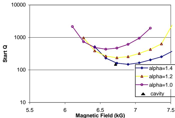
Fig. 3. Start oscillation curves as a function of average velocity ratio for the operating modes of (a) first harmonic cavities, (b) second harmonic buncher cavity, and (c) second harmonic output cavity. Curves plotted represent the threshold quality factors for a 100 MW beam as a function of axial magnetic field. Cavities which have quality factors that lie above this curve at a given magnetic field will be unstable to the operating mode.
