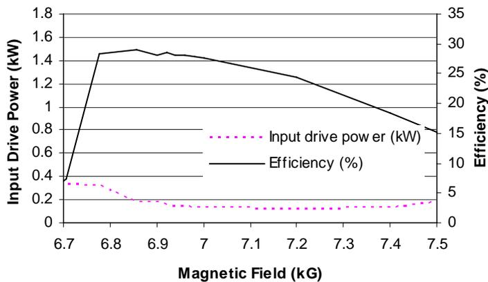
Fig. 7. Change in efficiency with change in magnetic field
