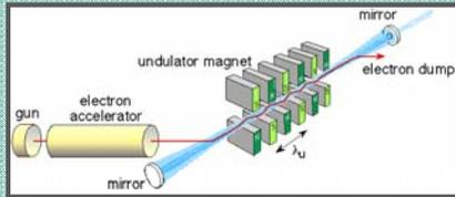
The FEL wiggler oscillates the beam through an alternating magnetic field.
