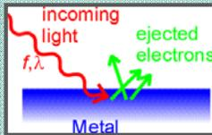
An important feature of photocathodes is **Quantum Efficiency (QE)**, the ratio of emitted electrons per incident photons:
