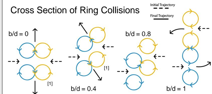
Also, velocity calculations have shown that little momentum is transferred for collisions outside the ring's diameter. Instead these collisions produce instability in the ring causing eventual vortex shedding and loss of momentum due to viscosity.
