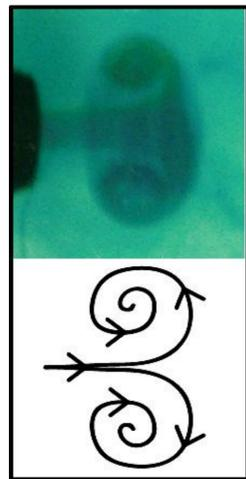
Vortex rings are characterized by their Reynolds Number, a dimensionless quantity which expresses the ratio of inertial and viscous forces. A ring with a Reynolds Number under 1000 is considered completely laminar.
