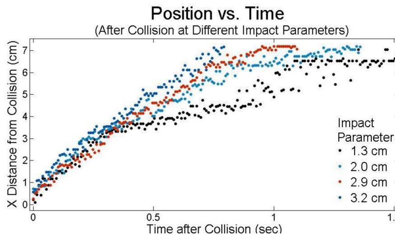
When the impact parameter is above 1.2 cm, the rings pass by each other becoming unstable with varying amplitudes. Immediately after collision, tests showed that rings all traveled with similar speeds no matter the impact parameter. But at later times, speed changed drastically. This is most likely due to the amplitude of instability produced from each collision. Scattering can also be observed in this stage.
