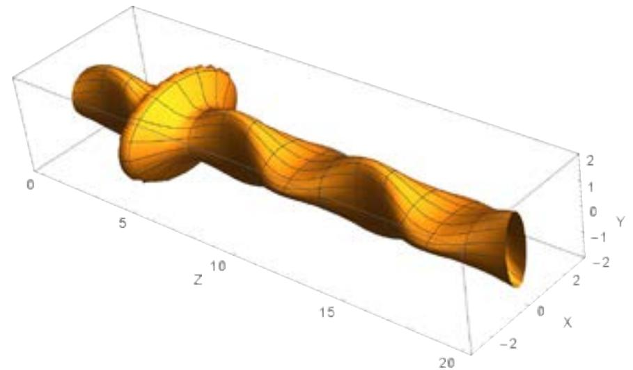
Fig. 5: This is a simplified 3D visualization of the beam. The bulge indicates altered shape in the injection line. The beam is squashed horizontally and vertically, alternating.
