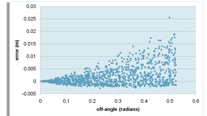
Top left: A simulation of the iterated formula for distance, charting the real distance versus the calculated distance, with the condition that the off-angle was less than 30 degrees.
