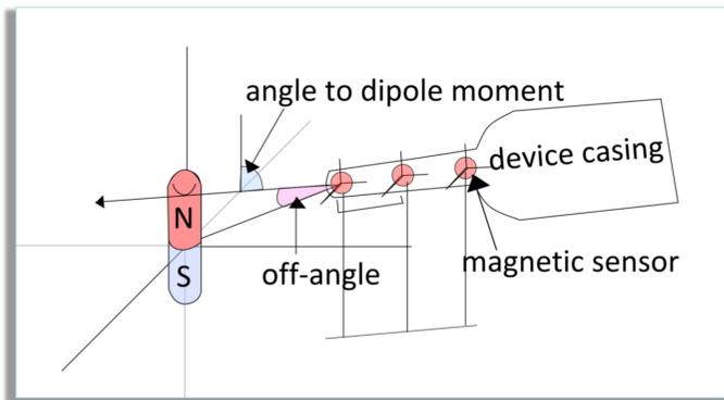
A diagram of the problem setup for the simulations, to clarify terminology. The lines on the sensors represent the axes where the magnetic field is measured,
