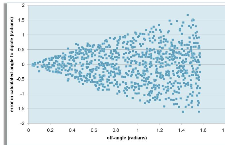
Left: A simulation of the iterated formula for angle to the dipole axis of the magnet. The maximum error in the calculated angle to the dipole increases as the off-angle increases, in a close-to-1:1 ratio.
