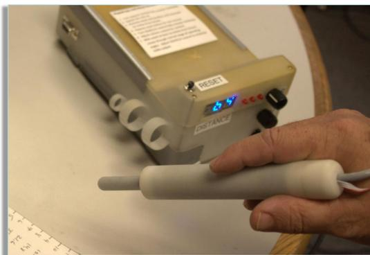
An early prototype of the device. The box shows the estimated distance to the magnet and emits beeps of varying frequency, depending on the estimated distance.
