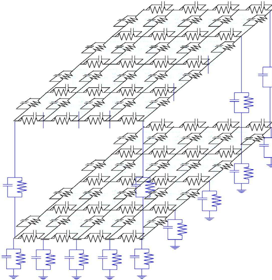
Only 5x5x2 mesh shown for simplicity. Not all vertical connections shown.
