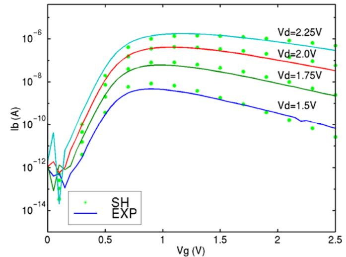
Using the new simulator to model EM induced avalanche breakdown
