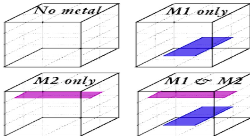
*Sample unit cells for a two-metal process*
