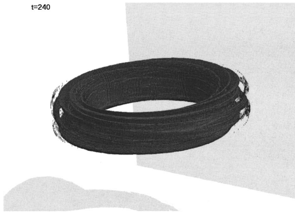
FIG. 7. Three-dimensional structure. The figure shows a surface of constant pressure during the nonlinear evolution of the \beta_{\text{pol}}=1 equilibrium, at t=240\tau_A .
