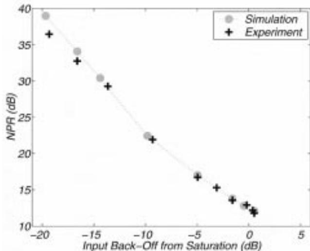
Fig. 6. Comparison between simulated and measured NPR in a Hughes 8537H TWT as a function of total input power. All the simulations were run with  $n_f = 13$ , and the values shown correspond to the average of 50 realizations. The saturation point corresponds to an input power of  $-11$  dBm.
