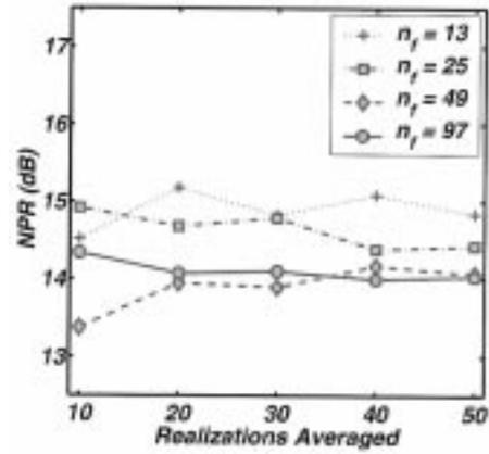
Fig. 3. Calculated NPR as a function of realizations averaged and size of frequency grid. The different symbols correspond to different number of frequencies as described in the insert. The bandpass is 36 MHz wide and centered at  $f_0 = 1.6498$  GHz, and the total input power is  $-16$  dBm.
