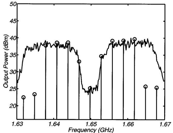
Fig. 7. Comparison between the time-averaged experimental output spectrum (solid line) and simulated average spectrum (50 realizations averaged, vertical lines with circles) for a total input power of  $-14$  dBm. The first and last two points of the simulated spectrum are below the experimental value because, on input, the amplitudes of these points are set to zero to minimize aliasing.
