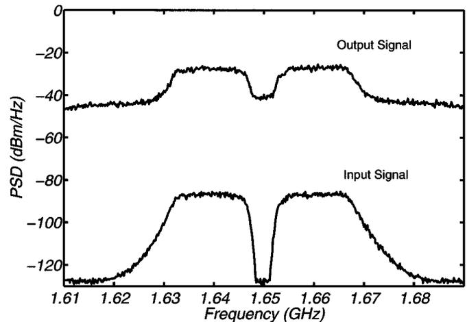
Fig. 5. Time-averaged input and output spectra for a NPR measurement with total input power  $-14$  dBm (3 dB input back-off from saturation, where saturation =  $-11$  dBm).
