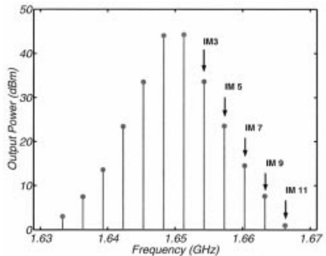
Fig. 9. Two-tone intermodulation products calculated with CHRISTINE.
