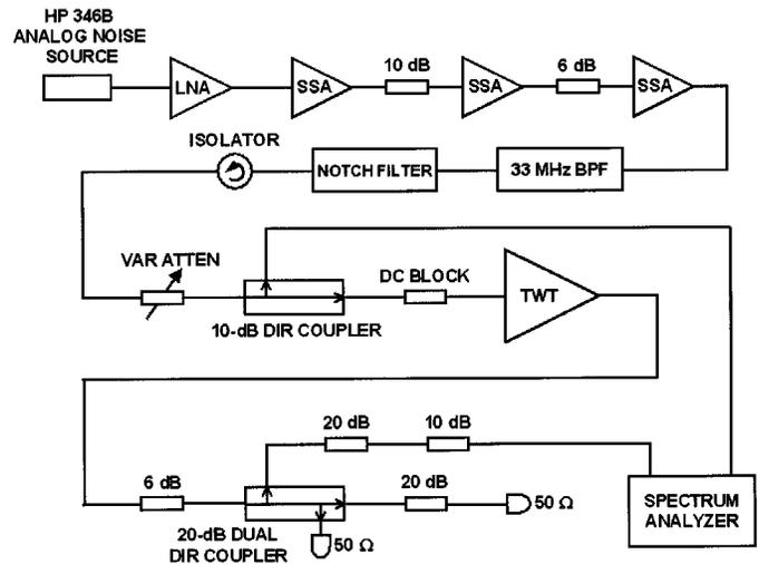
Fig. 4. Diagram of the experimental setup for measuring the NPR in a Hughes 8537H TWT.
