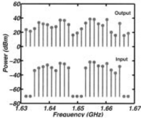
Fig. 2. A typical input and output spectrum for a run with 25 frequencies spanning a 36 MHz range centered at  $f_0 = 1.6498$  GHz and total input power  $-14$  dBm (3 dB input back-off from saturation, where saturation =  $-11$  dBm). The notch is covered by five frequency points, three at the bottom ( $s_j = 0$ ), spanning 3.0 MHz, and two at the  $-3$  dB points ( $s_j = 0.5$ ).
