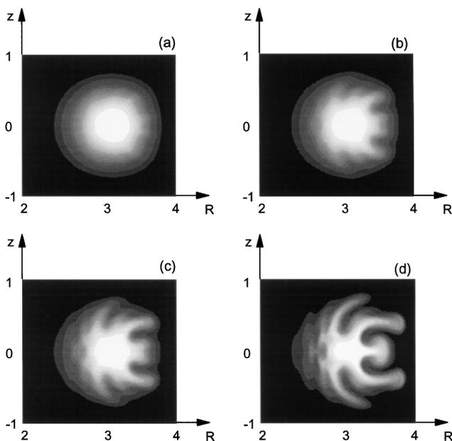
FIG. 1. Temporal evolution of the pressure in the poloidal plane ( $R, z$ ) at  $\phi = 0$  for a plasma with  $\beta_{pol} = 1.0$  and  $\eta = \mu = 3 \times 10^{-4}$ , at  $t/\tau_A = 0$  (a),  $80$  (b),  $120$  (c), and  $180$  (d).
