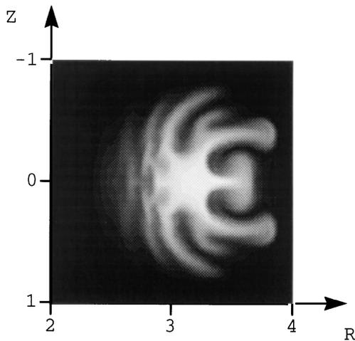
FIG. 4. Pressure in the poloidal plane  $(R, z)$  at  $\phi = 0$  for a plasma with  $\beta_{\text{pol}} = 1.0$  and  $\eta = \mu = 2 \times 10^{-4}$ , at  $t/\tau_A = 180$ .
