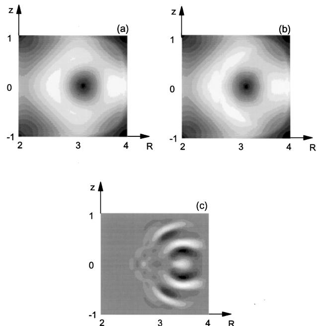
FIG. 2. Temporal evolution of the magnitude of the poloidal magnetic field in the poloidal plane at  $\phi = 0$ , at  $t/\tau_A = 0$  (a) and  $180$  (b). The momentum in the direction of the major radius at  $t = 180\tau_A$  is plotted in (c).
