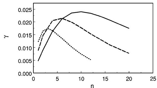
FIG. 3. Linear stability. The growth rate  $\gamma$ , normalized to the Alfvén time  $\tau_A$ , is plotted for modes with toroidal mode number  $n$ , for three different values of the resistivity:  $\eta = \mu = 1 \times 10^{-3}$  (dotted line);  $3 \times 10^{-4}$  (dashed line);  $1 \times 10^{-4}$  (solid line).
