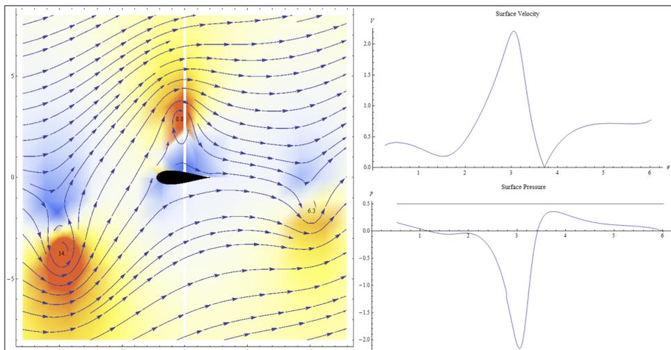
Surface velocity is calculated by taking the norm of the velocity vector at points on the fish's surface. Surface pressure is calculated by Bernoulli's equation for time-dependent potential flows:
