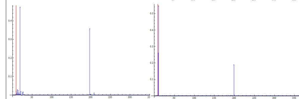
Posterior probabilities for the angle of attack after 1, 2, 4 and 8 time steps with 23 simulated velocity sensors on the surface of the fish with  $N(0, .25)$  noise, a freestream velocity of 1 and an 'unknown' angle of attack of  $9^\circ$  (shown as the red line).
