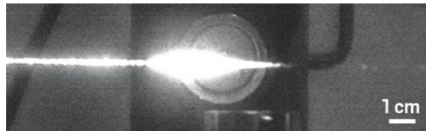
The plasma generated by Howard Milchberg's laser (traveling from the left) interacts with the free electrons in the air above a polonium-210 source.
